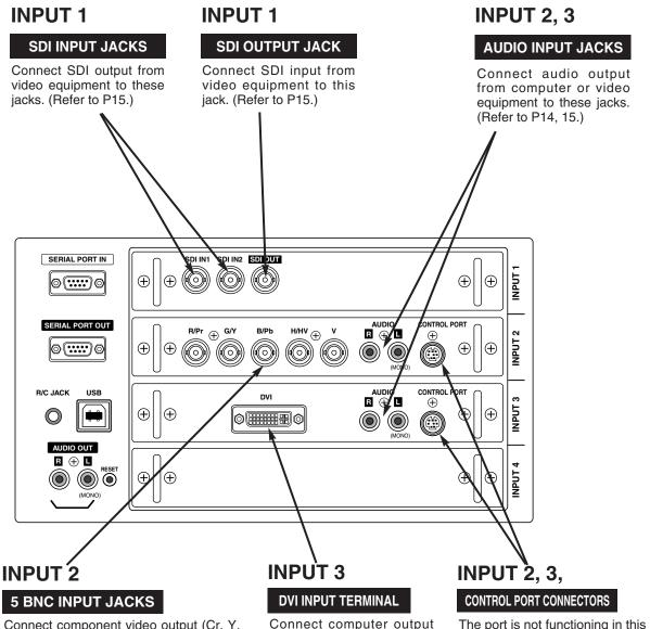
Connect component video output (Cr. Y. Cb or Pr, Y, Pb) from video equipment to R/Pr, G/Y and B/Pb jacks or connect computer output [5 BNC Type (Red, Green, Blue, Horiz. Sync and Vert. Sync.)] from computer to R/Pr, G/Y, B/Pb, H/HV and V jacks. (Refer to P14, 15)
